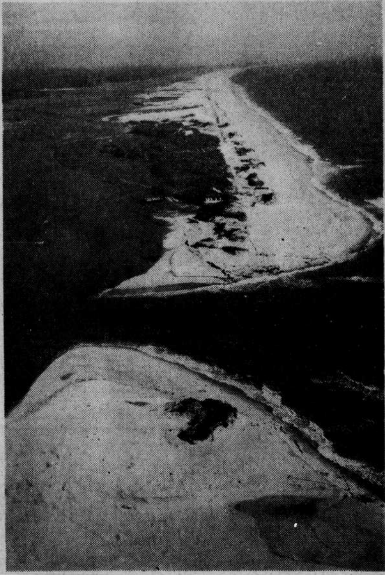
CLOSED—This is an aerial view of the inlet that cut across the lower end of Long Beach during Hurricane Hazel in the fall of 1954. Attempts to close this inlet proved futile until the USE Dredge Henry Bacon undertook the task about 6 weeks ago. Through the use of hydraulic fill, they have been able to erect a barrier against the sea and at the same time have joined once more the two beach areas.—Newton Photo.
