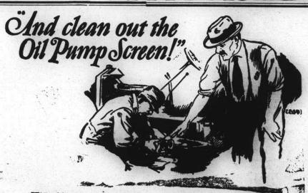
N addition to draining the old oil every 500 miles the experienced Fleet Boss insists on removing the crank case four times a year for thorough cleansing of the interior. He sees that the wire mesh pump screen is scrubbed with kerosene, for even partial clogging with dirt will keep oil from flowing evenly. Uneven pressure, no matter how good the oil, is responsible for many scored cylinders and burned out bearings.
