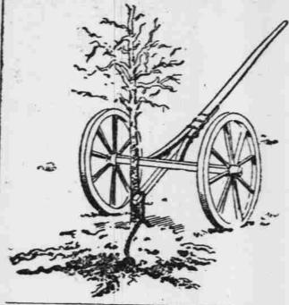
as the end of the joist attached to a chain that has been passed beneath the tree in two or more directions. When the pole is brought down, the tree is raised from its position and can be gently bent forward to the axle, secured there, and carried off to its new location.
