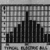
NOTICE how closely a typical customer's electric bill varied with the length of time artificial light is needed per day through the year.
