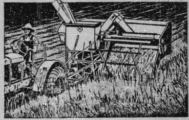
Above picture shows the new type "combine" reaper and thresher that has been bought by a group of Transylvania county farmers who are interested in growing small grains. The machine does the work of reaper and thresher all in one operation, and is said to be superior over use of both old types in salvaging grain, and is naturally a much cheaper outfit to operate, doing away with the "double trouble" of reaping, stacking, hauling, and threshing.
