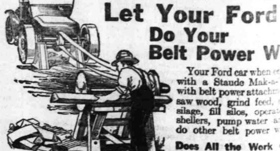
Belt Power Work Your Ford car when with a Staude Mak-awith belt power attaching saw wood, grind feed, and silage, fill silos, operate
