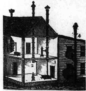
Our Fire Clay Chimney Pipe does not rust for crack by heat nor crumble from frost, It has been used ten years for dwellings, schools churches &c. No danger from fire as it does not communicate heat to wood. Insurance Companies have decided it to be a safer chim-ney than brick. Any one can put it up. We show four forms of constructions. A com-plete chimney costs from \$5 to \$10 according to height of building. Ar Send for descriptive circular with full information.
