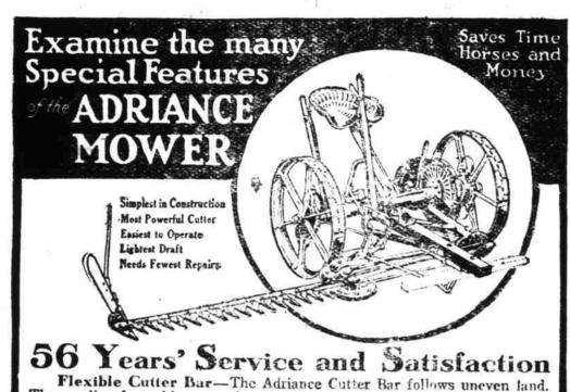
The coupling frame hinges are in exact line and swing like a door-no binding. The bar can be folded over the tongue when not in use. Knife Starts Instantly—The clutch is on the high speed shaft—thus starting the knife instantly and avoiding clogging. The driving pawls are also
