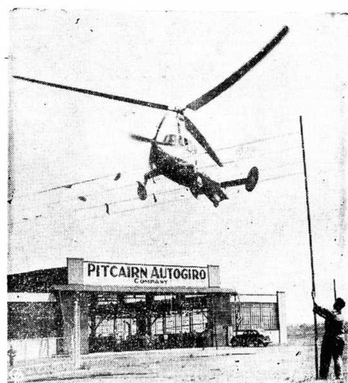
First showing of the new PA-36 autogiro is staged at Pitcairn Field, Harbor, Pa., for benefit of army and navy observers. Pictured soaring over a ribbon hazard, the machine can rise vertically, needs no runway.
