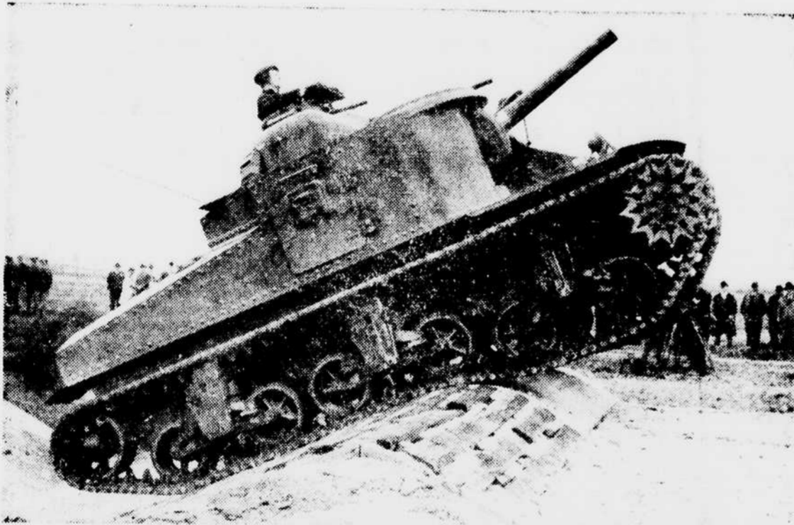
Tested at Aberdeen, Md., is the Army's new 25-ton tank, said to be the most powerfully armed machine of its type in existence. The traveling fortress is armed with a 75-mm. and a 50-mm. cannon and five .30 calibre machine guns. The Army is building large numbers of these tanks.
