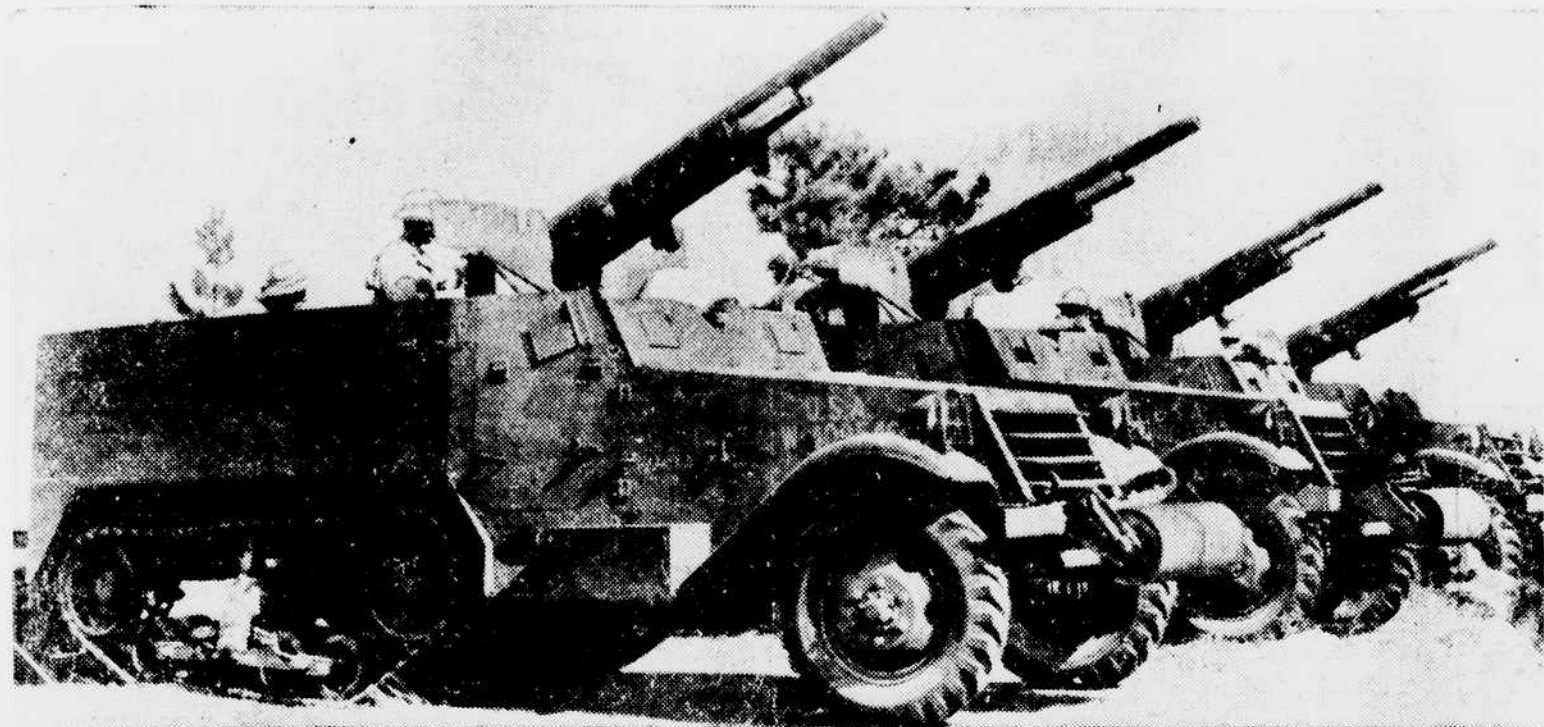
Mechanized equipment of the First Armored Division from Fort Knox, Ky., known as "Old Ironsides" is lined up for battle practice at Rock Hill, S. C., in the Army's huge war maneuvers. The vehicles are half-truck, half-tractor, serving as a mount for the highly efficient 75 mm. field piece. Not seen are the ammunition trailers which are pulled by the tractor-trucks. (Central Press)
