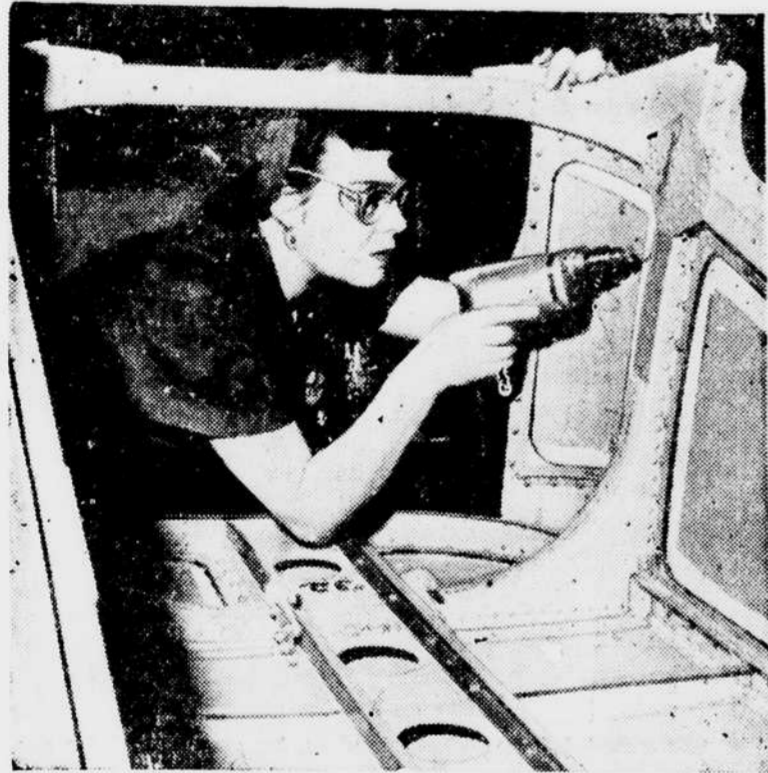
Mrs. Evelyn Casola, widowed by the Jap attack on Pearl Harbor, is getting back at the Nipponese by helping to build bombing planes at a big aircraft plant. She is shown drilling rivet holes in the fuselage of a U. S. bomber. (Central Press)
