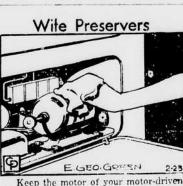
Keep the motor of your motor-driven home appliances clean. Excess dust may be removed with a cloth, or by blowing out the motor with a hand bellows, or with a blower attachment of an electric
