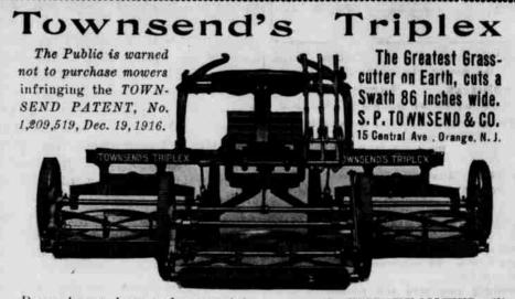
Drawn by one horse and operated by one man, the TRIPLEX MOWER will mow more lawn in a day than the best motor mower ever made, cut it better and at a fraction of the cost.
