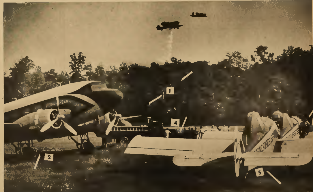
QUITE A PROJECT —Putting "Water Bomb" planes into the air to fight forest fires at Tri-County Airport, Tuesday, meant need for plenty of equipment. No. 1, shows target—two trees and above the lead plane has just signaled the target and plane 2 is dropping 350 gallons of water. Below, left, the big DC-3 gas tanks are fueling one of the planes with No. 2 pointing to the electrical equipment on
