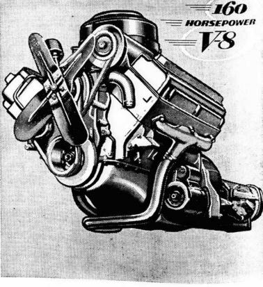
FIRE DOME has famous dome-shaped combustion chambers with centralized spark plugs ... the engine design that gets more power from every drop of gas. This new De Soto will be the most talked about car of 1952. See it TODAY!
