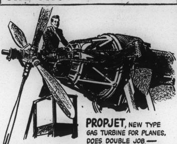
TURNS THE PROPELLER AND ADDS POWER THROUGH A JET TO THE REAR. EXPERTS SAY PROPJET WILL POWER GIANT TRANSOCEANIC AIR LINERS OF TOMORROW. IT WAS DESIGNED BY GENERAL ELECTRIC ENGINEERS.
