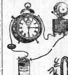
A sure cure for oversleeping, as the Electric Bell rings until the Swith opened and this can not well be without getting out of bed, as it be located at any point in or out of room.
