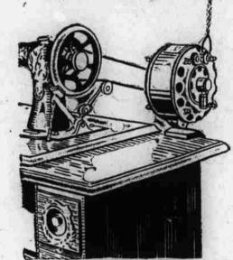
Gemotor Attached to Sewing Machine
