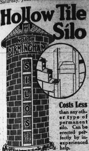
Tiles are curved to form a perfect circle. Grooves in tiles hold tie wires all around, covered with concrete mortar—forming a solid, wind-proof, fire-proof, crack-proof, acid-proof wall. Hollow spaces in tiles keep silage in best feeding
