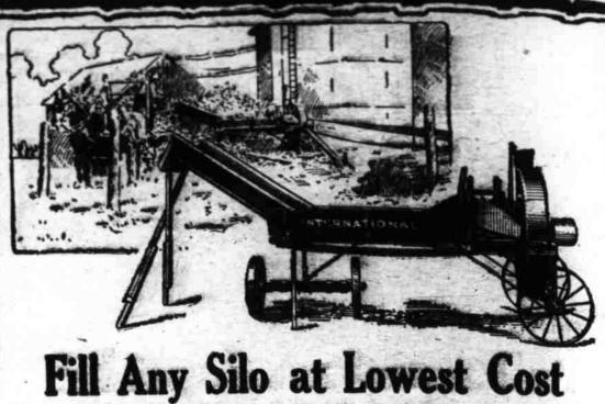
INTERNATIONAL Ensilage Cutters now made in five sizes, with capacities ranging from 3-6 to 16-25 tons per hour. The line now includes sizes for filling every silo, from the smallest to the largest and highest.
