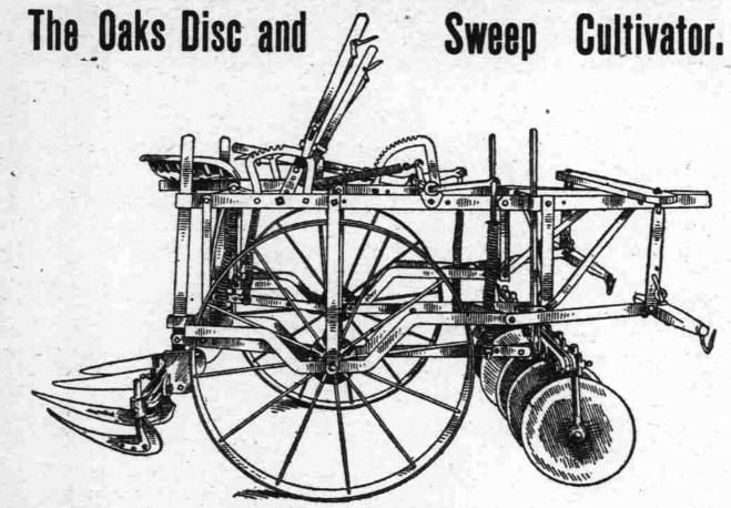
This cultivator is especially designed to meet the requirements of the cotton and corn grower, with discs in front and sweeps in the rear. Relief springs are attached to both discs and sweeps in case of stumps or stones. The adjustments are set on steel sliding bars so as to enable one to work any row from 3 to 5 feet wide, leaving the land in perfect condition, taking out all the middle. Write for free circular and prices. THE OAKS MANUFACTURING CO., New Bern. N. C.
