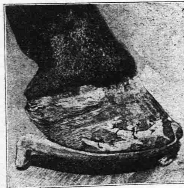
Fig. 11.—This illustrates a poor job of clinching and finishing a foot
