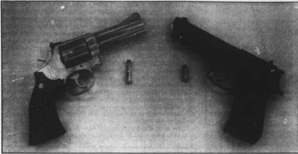
The Smith & Wesson .357 magnum revolver (left), carried for years as the standard equipment of N. C. Highway Patrol officers, has been replaced by the Beretta 9mm automatic pistol (right). The new weapon carries 16 cartridges as
