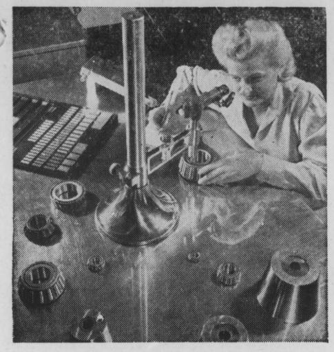
Imagine a table so smooth that flat objects cannot be picked up but must be slid off the side and you have an idea of this table used in the tool inspection department of the Timken Roller Bearing Company. Finished to within fifty one-millionths of an inch for flatness, the table is kept in an air-conditioned for the greatness possible accuracy in measurement readings. About the only use we can think of in Zebulon is for the loan table Vance Brown puts money on at the local bank.
