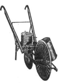
Most perfect furrow opener on the market. Automatic throw-out device is patented and possesses many advantages not found on other planters. Flat and edge drop plates with each planter. Two, three or four kernels to the hill without changing plates. Features that are of vital importance to the corn grower.
