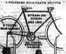
Note tht enormous increase in the strain smaller sprockets and a 9-inch lower gear.
