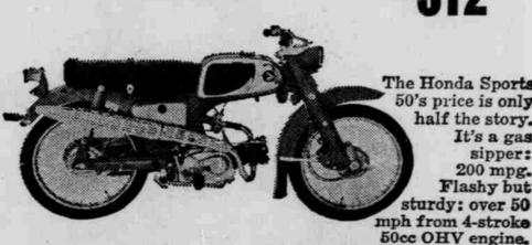
Flashy but sturdy: over 50 mph from 4-stroke 50cc OHV engine. Other virtues: 4-speed transmission, manual clutch, camtype brakes. Sheer fun to own.
