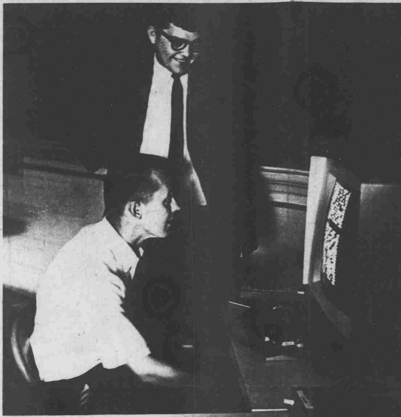
NO, THIS is not a television, it's an IBM 2250 Graphical Display Device. Staring at it in disbelief is DTH News Editor Don Campbell. When news copy appears in the screen, you point the light gun at a mistake, press a button and a pedal and the mistake disappears. See the story below to find out what else it does. —DTH Photo by Steve Adams
