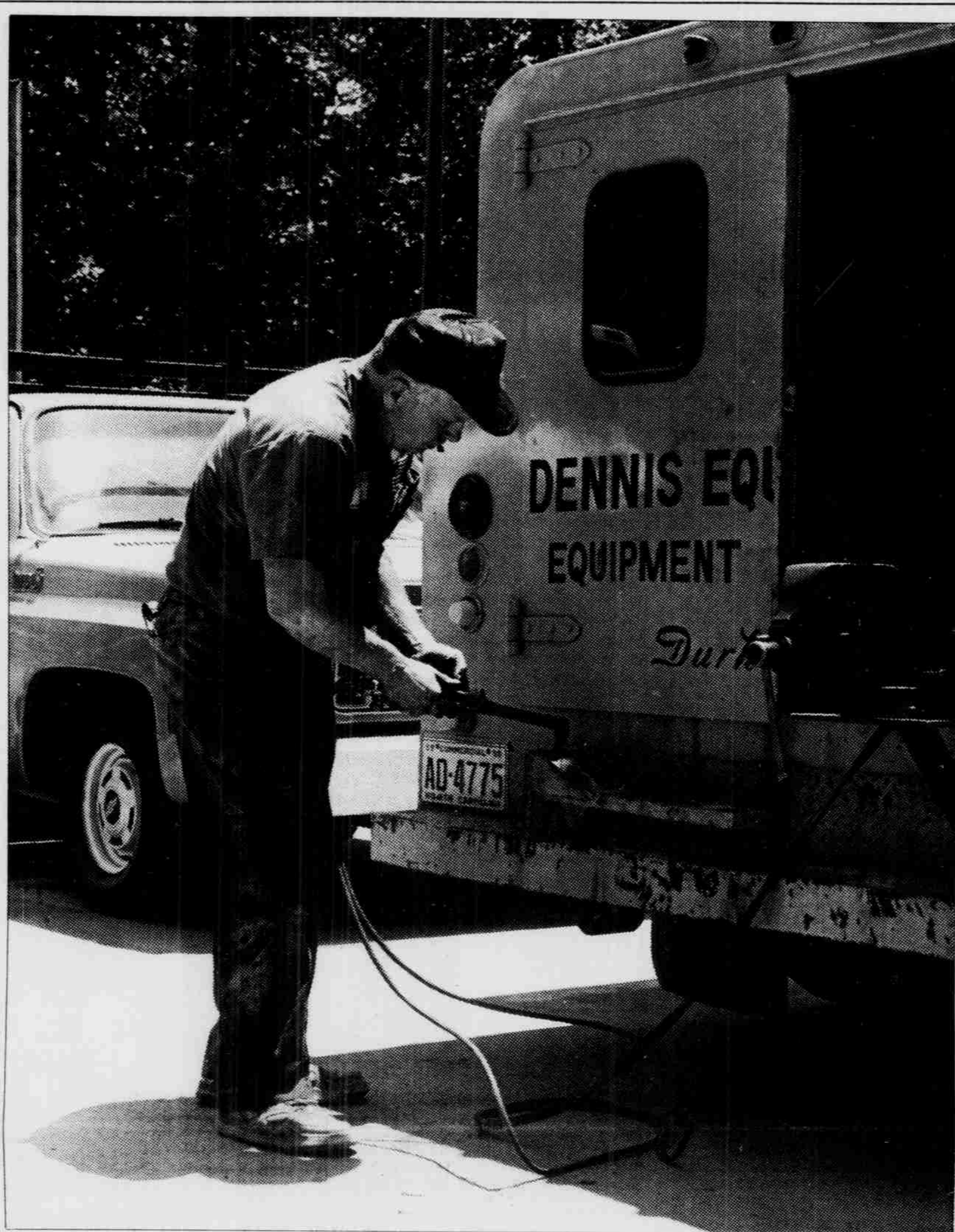
Flame on Alan Forthofer of Dennis Equipment Rental uses an oxyacetylene torch to weld a part Tuesday afternoon in the parking lot near the unfinished Alumni Center on Stadium Drive. DTH/Dave Layton
