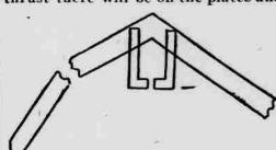
ROOF TRACK FOR HAY CARRIER. he easier will the load be carried. Rafters two by six-inch will be strong enough to carry an ordinary barn roof and the load of hay, since the track is attached to every pair of rafters, and the rafters are but 16 inches apart. This distributes the load. If the barn is small and the roof steep, two by four-inch rafters will be strong enough. The steeper the pitch the smaller the rafters may be, other things being equal.-Country Gentle-
