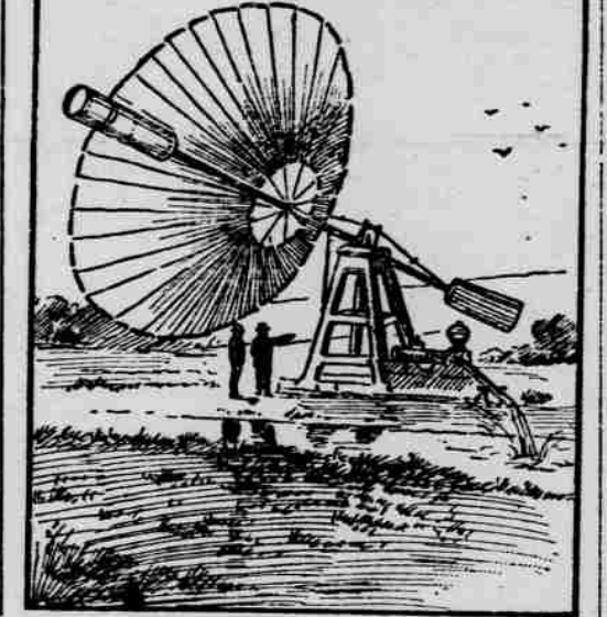
MODERN SUN REFLECTOR. (Used in California for Heating Water in Boilers and Tanks.)
