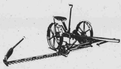
Years of service lie ahead for the McCormick-Deering No. 7 Enclosed-Gear Mower. The entire operating mechanism, including the drive gears, differential, and countershafts, is assembled compactly in an oil tight gear housing and runs in a bath of
