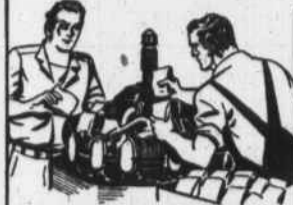
U. S. INDUSTRY HAS DEVELOPED A CHEMICAL DEHYDRATOR TO PACK (IN BAGS) WITH AIRPLANE MOTORS DURING SHIPMENT TO OUR FIGHTING FORCES OVERSEAS BY MAKING IT UNNECESSARY TO COVER ENGINES WITH GREASE IT SAVES 100 MAN-HOURS OF CLEANING.
