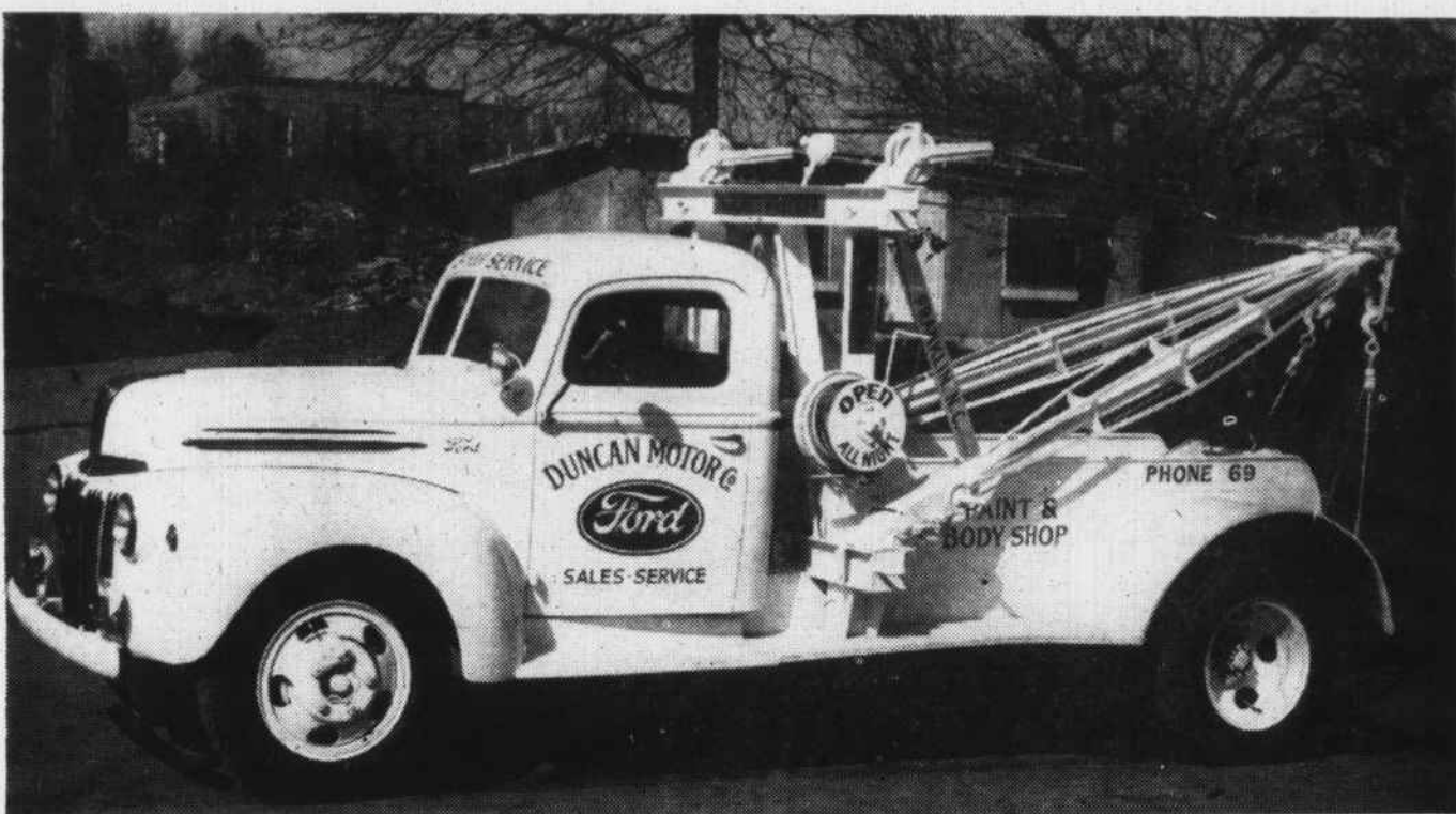
DAY AND NIGHT WRECKER SERVICE —Duncan Motor Company operates a 24-hour Wrecker Service, and the photograph above suggests how well equipped it is for that service. The picture is of a 1946 Holmes Heavy Duty Wrecker, mounted on a new Ford chassis, recently put into service by the Duncan Company. This wrecker, being heavy duty equipment, enables Duncan Motor Company to handle the big wrecks, as well as the smaller ones. It's wrecker service is available at any hour. (Adv.)
