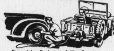
Power take-off at rear of "Jeep" can be used to operate air compressor unit.
