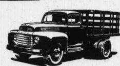
F-5 STAKE—New Ford <u>Bonus Built</u> Stake is available in 9 ft. and 12 ft. lengths. 14,000 lbs. G.V.W. Choice of two truck engines . . . a new 95 h.p. six-cylinder engine . . . or a new 100 h.p. V-8. Quadrax rear axle. 2-speed rear axle available on Series F-6.
