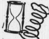
HOURL-GLOSS COILS—Self-equalizing; prevent mattress "slope."
