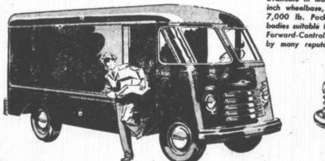
FORWARD-CONTROL CHASSIS Model 3942—137-inch wheelbase, Maximum G.V.W. 10,000 lb. Also available in model 3742—125 1/4-inch wheelbase, Maximum G.V.W. 7,000 lb. Package Delivery type bodies suitable for mounting on the Forward-Control Chassis are supplied by many reputable manufacturers.
