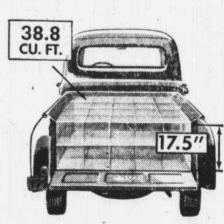
7 cubic feet MORE payload than the other leading make of Pickup! Supported load capacity of the other leading Pickup is only 31.6 cu. ft. The FORD Pickup gives you a full 38.8 cu. ft.! . . . space for extra cartons or crates, and the 3-inch higher side panels let you haul bulky or unstable loads with more ease and safety.
