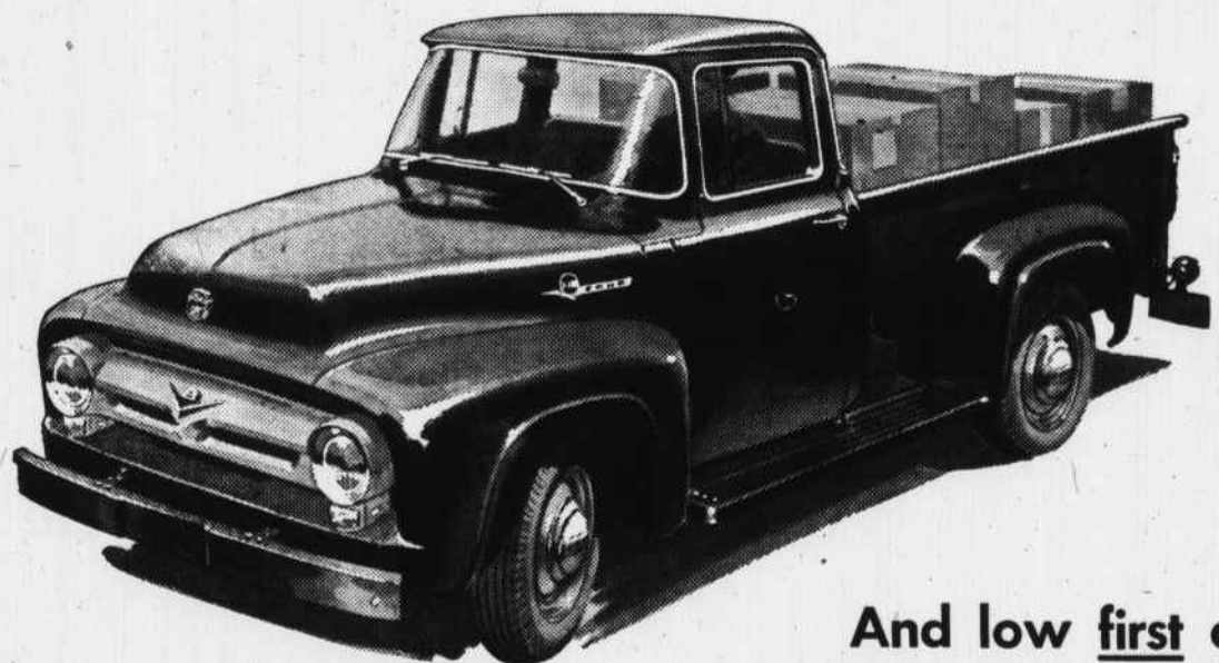
Ford's F-100 pickup with 8-ft. box is the biggest in the half-ton field—up to 19 cu. ft. more loadspace than the others. Regular 6 1/2-ft. box with a full 45 cu. ft. capacity also available.
