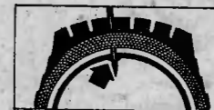
Seals with nail in. Self-healing lining closes around the nail . . . blocks escape of air.
