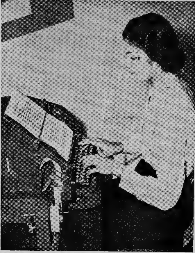
Pretty Betty Ruth Boyd, of Monroe, N. C., is shown operating the keyboard of a Teletype-setter perforator, the machine that has opened up an entirely new occupation for women in the newspaper field. The tape from this machine (shown in the lower left hand of the picture) is fed through an apparatus attached to a typesetting machine and automatically sets type for newspapers. Miss Boyd is a student at the Roy Parker School of Printing, Chowan College, Murfreesboro, N. C., the only school in the entire South where such training is available. (Chowan College News Bureau Photo.)
