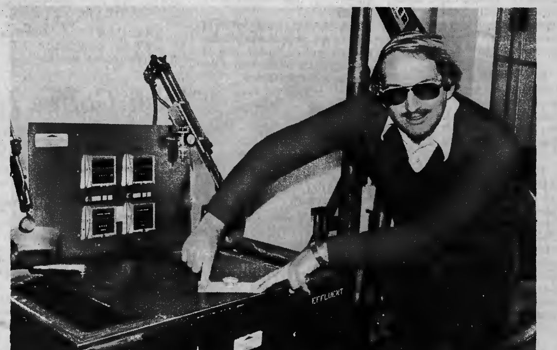
READY FOR THE CREEK — Gary Frick, superintendent of the Moore County Water Pollution Control Plant, shows a sample of the plant's finished product, known as effluent. Once raw sewage, this water has been treated and cleansed of pollutants and is ready for discharge into Aberdeen Creek. The equipment is an automatic sampler which scoops up a tiny cup of water every five minutes for continuing monitoring.
