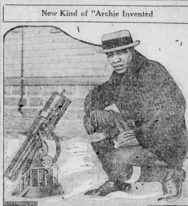
Robert Blair of Detroit with the new type anti-aircraft gun which he designed. Its special feature is an electric searchlight finder. The War department is interested in this newest development of defense against air attack.
