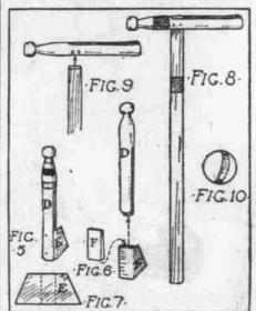
made with a clothespin (D), a cardboard shoe (E), and a small wooden wedge (F). Cut wedge F to fit the open end of the clothespin, and after cutting the cardboard shoe E by the pattern of Fig. 7, fold it as shown in Fig. 6, tack to the edges of wedge F. and slip into the open end of the clothespin as shown in Fig. 5. Then drive a couple of tacks through the clothespin into wedge F.
