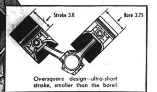
Here's the measure of a truly modern V8 engine—Chevrolet's advanced oversquare design. It means less friction...longer engine life!
