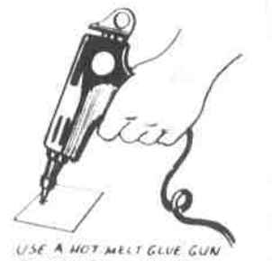
USE A HOT MELT GLUE GUN TO MOUNT THE PHOTOS. THE GLUE IN A NEW GUN MADE BY LABELER SETS IN 20 SECONDS, WHILE THE HANDY STAIN! PALKA WITH LACER GUN! ALLOWS THE USE OF BOTH HANDS FOR POSITIONING THE PHOTOS.
