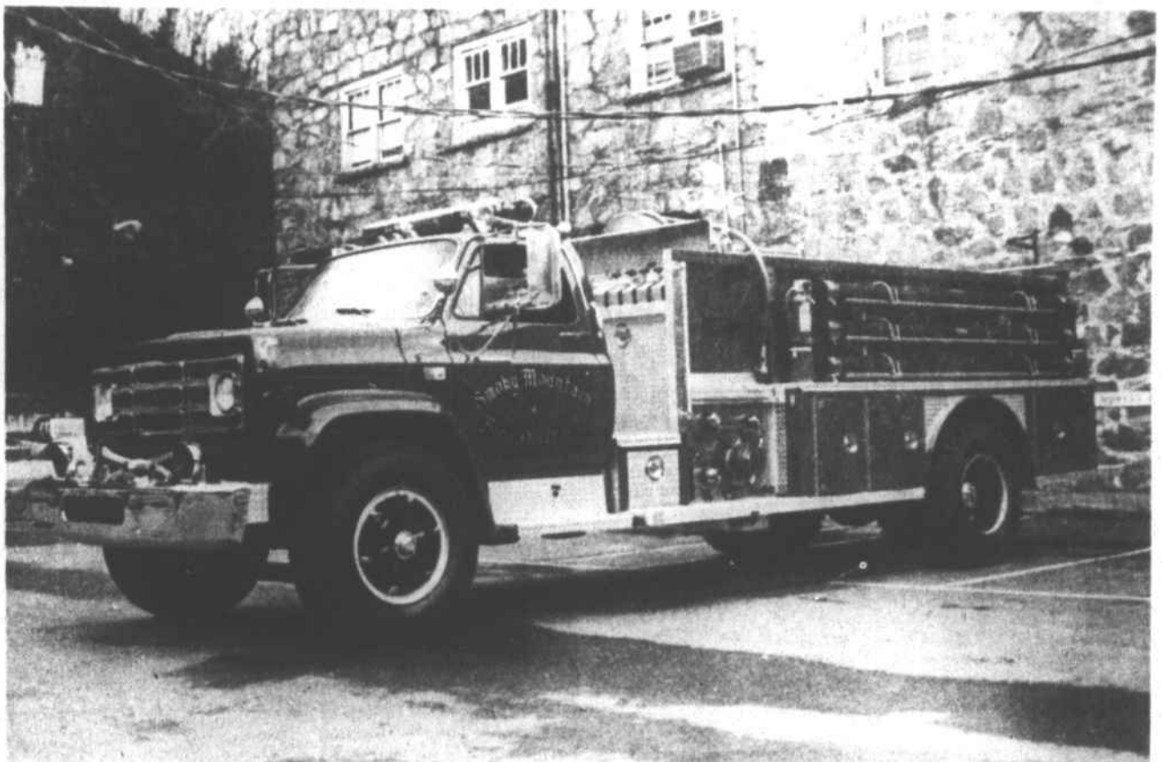
MARSHALL'S NEW FIRE TRUCK arrived in town last Friday from Columbia, S.C. The truck, an all-aluminum emergency one body on a 1980 GMC chassis, has a 1,000-gallon tank capacity and a special 1,500-gallon portable folding tank.
