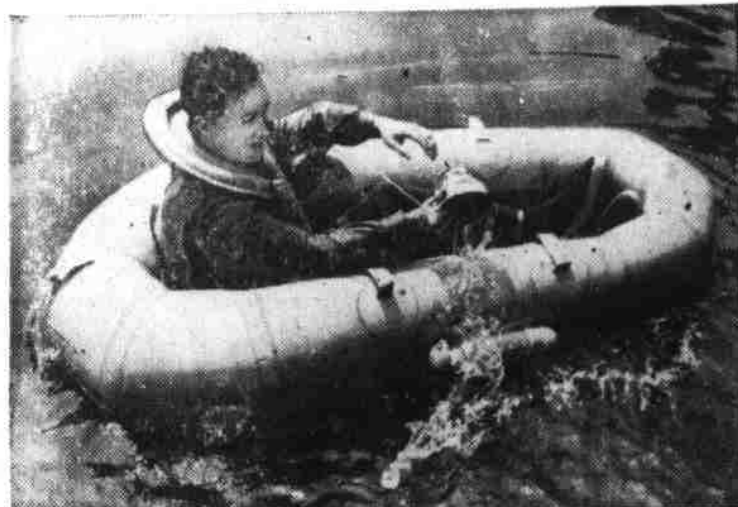
Demonstrating a new one-man rubber boat for use in fighter planes is Ralph Douglas. He is shown bailing out some of the water that splashed into the rubber lifeboat while he was inflating it in the East River in New York City. The boat can be inflated almost instantly by a pilot forced down in water and weighs only twelve pounds. It is carried in a small pack on the flier's back. (Central Press)
